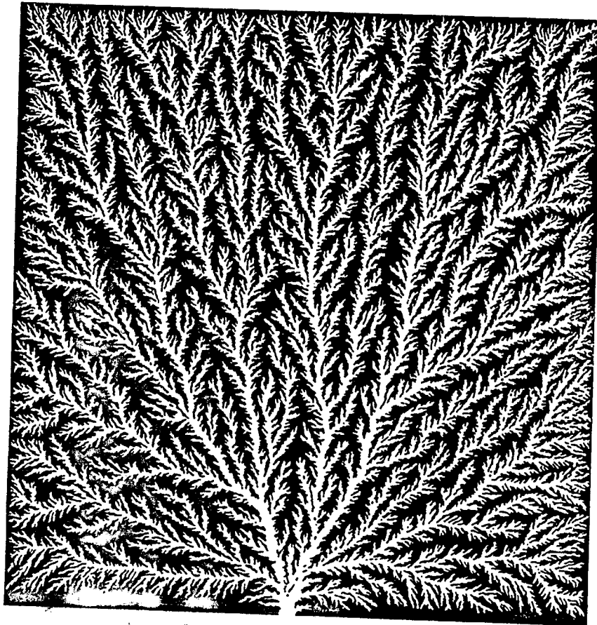
A positive Lichtenberg figure, obtained when a block of plastic is charged with static electricity.
